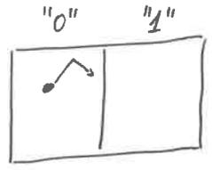
the particle can be on the left ("0") or on the right ("1") side of the box, representing one bit of information.
