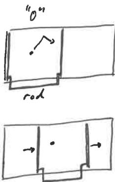
1. Insert two separators, in the middle and on the left edge. Connect them with a rigid rod.
